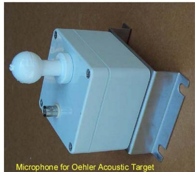
Each target is designed to use up to sixteen microphones. Full system capability requires use of all microphones. If the system need not solve for elevation and azimuth of incoming projectiles, local speed of sound or vector wind at the target, then the number of microphones can be reduced.
