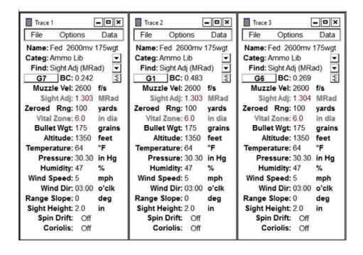
Examine the time-of-flight of the three traces. Trace 1 is the "truth" as described by G7. The times are similar for short ranges, but diverge for longer ranges. Note significant differences between G1 and G6.
